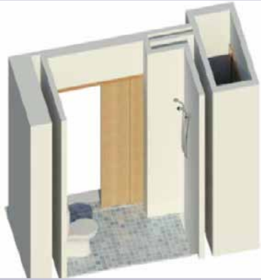
Figure 5. Merging the Shower and Toilet Spaces Reduces the Floor Area in a Small Unit
